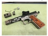
3. Remove the original compensator if installed from your upper receiver using an appropriate tool, FYI it is not necessary to remove the upper receiver from the lower frame assembly as shown in fig #2
